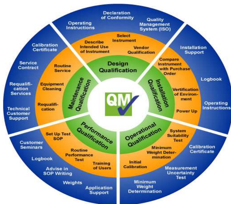
Fig. Equipment DQ, IQ, OQ, PQ and Maintenance cycle
